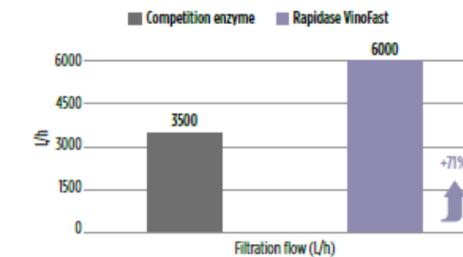
**Figure 3.** Filtration flow in a challenging thermoflashed red hybrid wine from the 2023 harvest with 2.2 mL/hL of Rapidase Vinofast. Added during AF, followed by a 2-month contact time (Canada, 2023).
