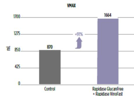
**Figure 2.** Vmax for red grapes with 30% *Botrytis cinerea*. Rapidase GlucanFree during AF at 3 mL/hL + Rapidase Vinofast after MLF for 1 week at 3 mL/hL. VITEC (Spain), 2025.
