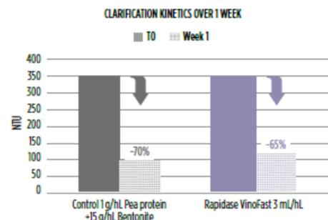
**Figure 1.** Clarification performance with 3 mL/hL of Rapidase Vinofast (without fining agents) versus control (with fining agents). Contact time: 1 week at 15 °C. Excel Ibérica (Spain), 2024.
